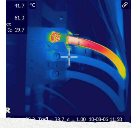
Electrical Safety - Worn our parts and loose connection leading to fire and/or thermographic hot spot or both. Due to overloading
